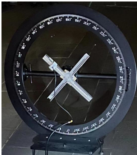
Figure 3. Schematic diagram of non-magnetic rotary table
