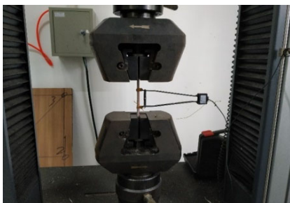
Figure 3. Tensile properties test
