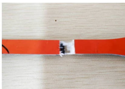
Figure 7. Fracture morphology of composite materials
