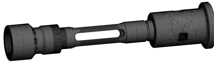
Figure 4. Solid mesh model of central pipe and upper joint
