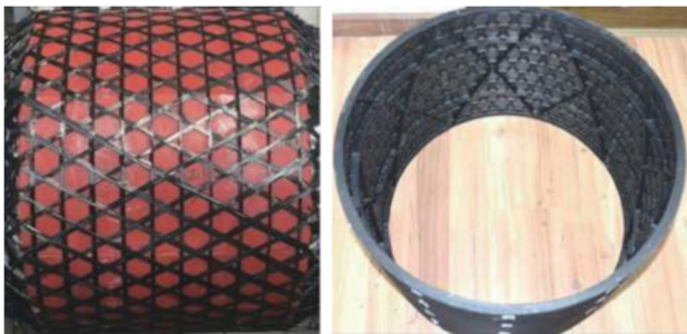
Figure 12. Hierarchical Kagome stiffened cylinder
