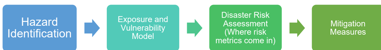
Figure 2. A flowchart visualising the process of natural hazard risk assessment and where risk metrics come in
