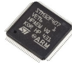
Figure 5. STM32F407 micro controller
