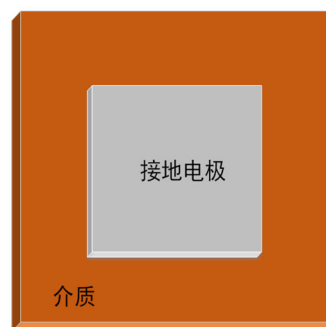
Figure 6. Structure of a dielectric-metal ground electrode
