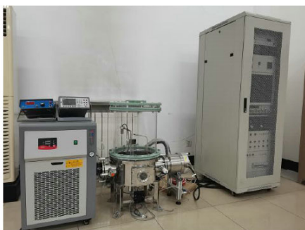
Figure 5. Vacuum system of low-pressure along-surface flashover test platform
