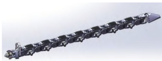
Figure 9. Snake pipeline robot
