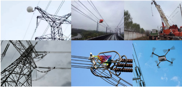
Figure 5. Transmission line foreign body invasion situation
