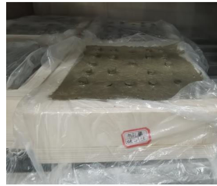
Figure 3. Specimen in constant temperature steam curing
