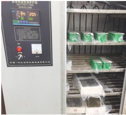
Figure 2. Constant temperature steam curing box for concrete
