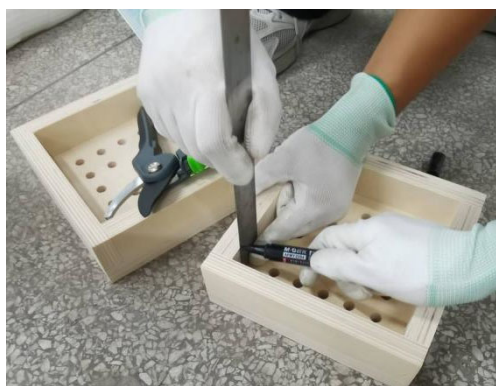
Figure 1. Test block size (150× 150× 30 mm)
