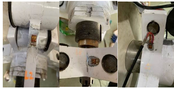
a. Connecting rod b. Small hub c. Large hub Figure 6. Load test measuring point layout.
