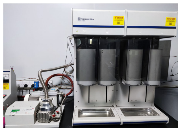
Figure 1. Physical diagram of the low-temperature N 2 adsorption experimental instrument.
