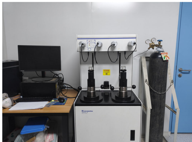
Fig. 2 High-pressure mercury intrusion porosimetry instrument physical diagram.
