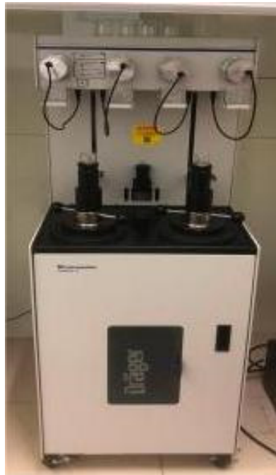
Figure 2. Fully automated pressure pumping pore size analyzer AutoPore V 9620
