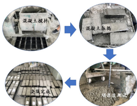
Fig 2. The pouring process of the test block
