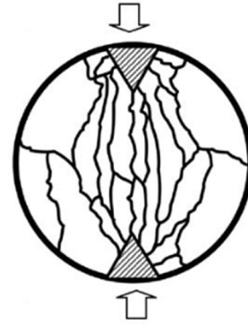
Figure 6. 3D schematic diagram of the crack pattern inside the sphere under impact load
