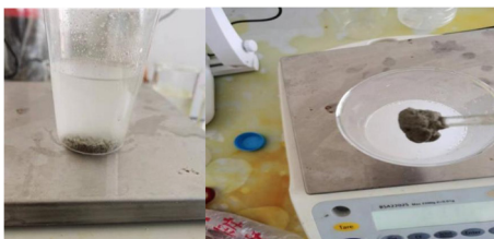
Figure 3. Bonding of the agent to the formation sand
