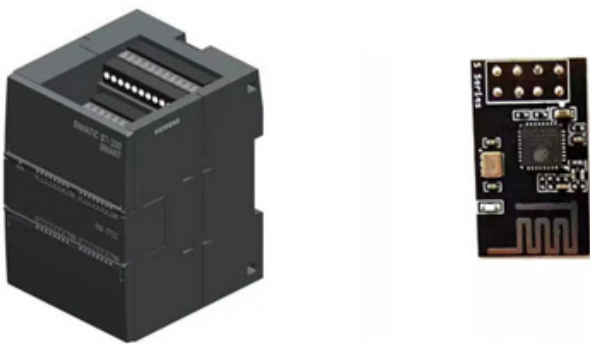
Figure 1. PLC processor (a) and WIFI module (b)
