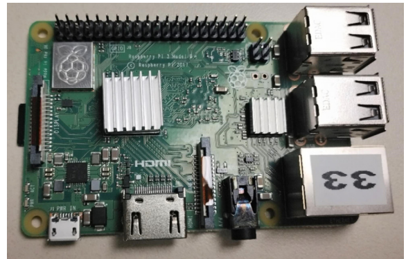
Fig 3. Raspberry Pi Model B+ used in our ambient sensor setup, facilitating seamless integration for elderly care assistance and activity tracking
