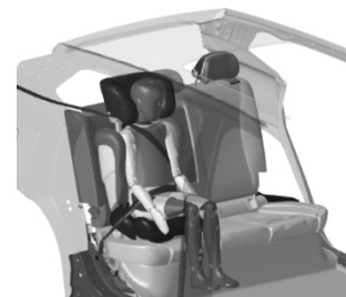
Figure 4. Simulation Model of the Q10 Child Dummy under MPDB Conditions
