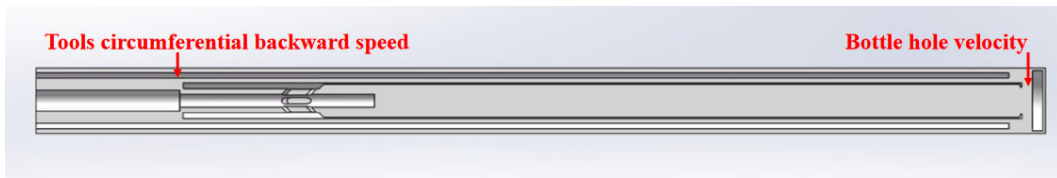
Figure 1. 3D model of coring tool (Taking \Phi 172 as an example)
