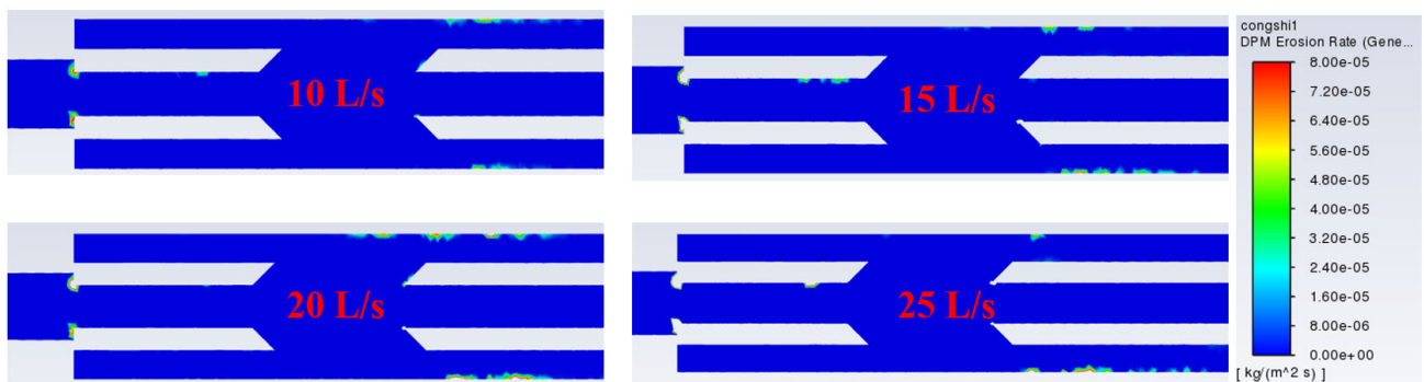
Figure 6. Erosion distribution of a \Phi 140 coring tool
