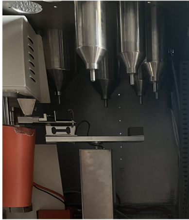
Figure 9. Powder discharging site of automatic batching machine
