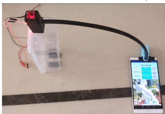
Figure 1. Schematic diagram of principle and finished prototype of smartphone spectrometer
