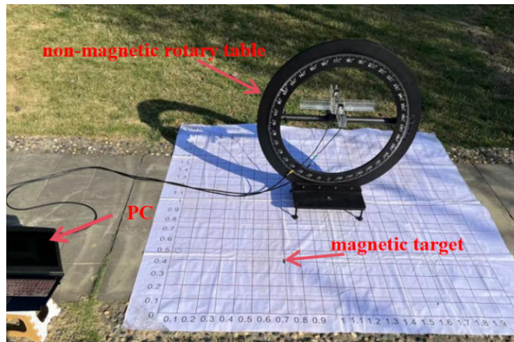
Figure 8. Magnetic gradient tensor localization system
