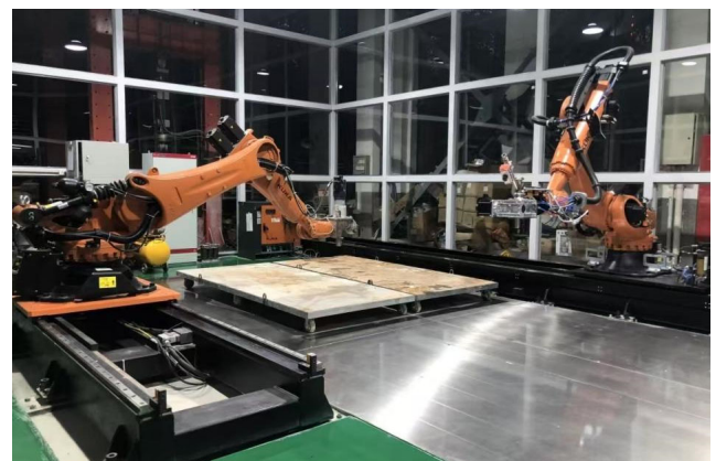
Figure 2. The robotic arm set up for printing
