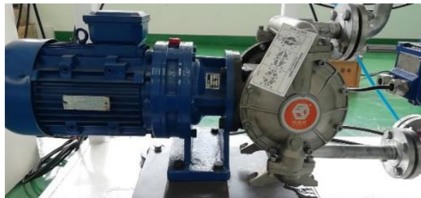
Figure 16. Electric Double-Cylinder Single-Acting Diaphragm Pump
