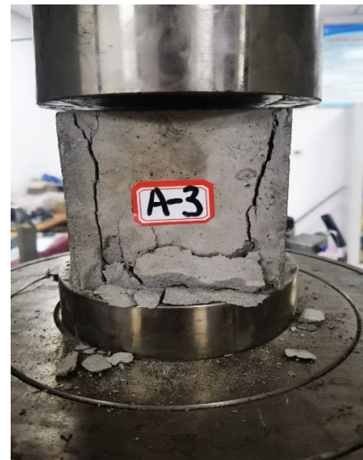
(b) Uniaxial compression test in laboratory
