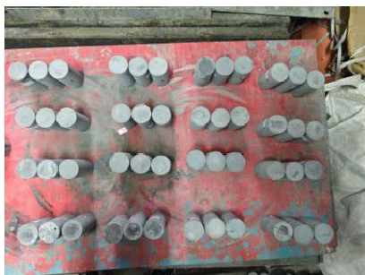
Figure 2. Rock Mass Mix Ratio Experiment
