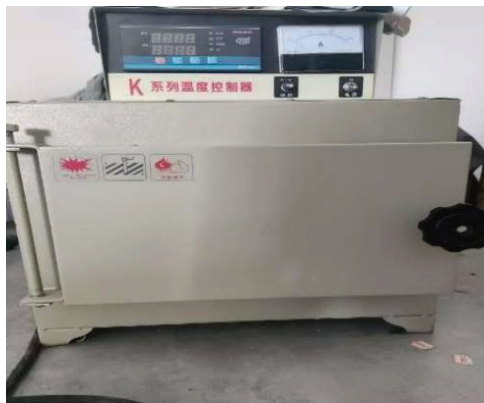
Figure 5. SX2-4-10 box-type resistance furnace
