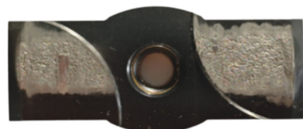
Figure 14. Wear state of the second guide pad
