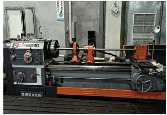
Figure 11. CW6163D deep hole drilling machine and workpiece
