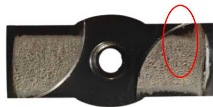
Figure 13. Wear state of the first guide pad
