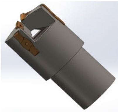
Figure 6. Simplified 3D model of BTA deep hole drilling tool
