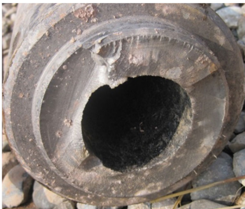
Figure 1. Failure diagram for drilling tool joints
