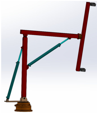
Figure 2. Schematic structure of diagram of the three-dimensional the well dressing machine's pipe-grabbing robot arm
