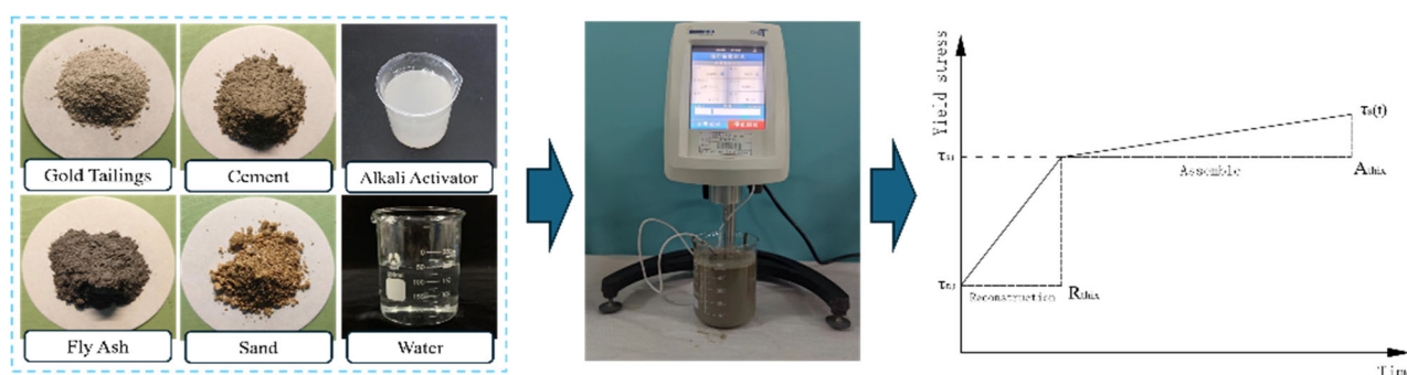
Figure 3. Measurement Process of Rheological Characteristic Curves
