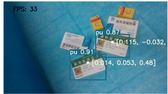
Figure 8. The effect of obtaining the 3D coordinates of the pill box
