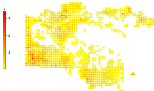
Figure 2-6. Grid distribution of total refrigeration space
