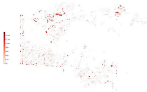
Figure 2-2. Spatial distribution of building unit refrigeration load
