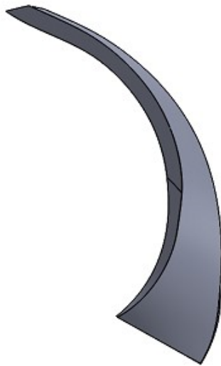
Figure 9. 3D solid model of a single twisted blade
