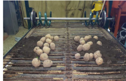
Figure 8. Separation device combining spring-type mixer and conveyor chain
