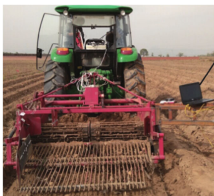
Figure 9. The installation positions of camera and potato harvester
