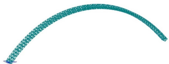
Figure 2.1 Finite element calculation model diagram of the main arch ring of the strong skeleton
