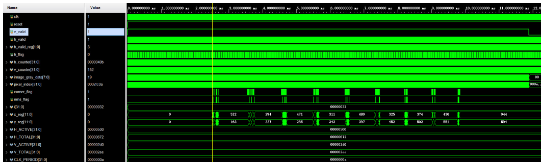
Figure 4. Simulation waveform diagram of the fast feature-detection circuit
