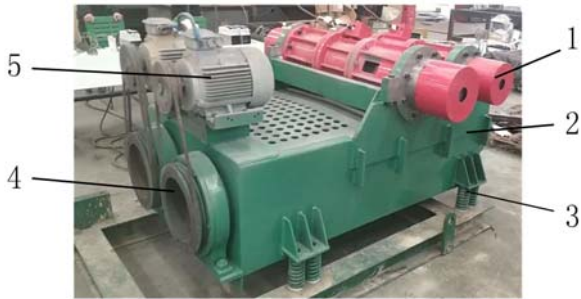
Figure 1. Structure of solid-liquid separator. 1 Vibration motor, 2 Box, 3 Damping spring, 4 Screen cylinder, 5 Pulley.
