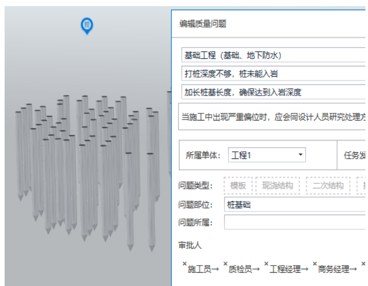
Figure 6. Pile Foundation Quality Control
