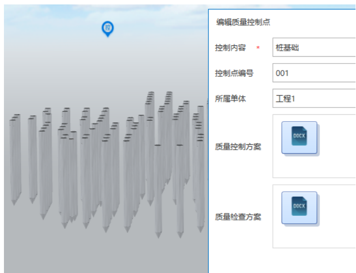
Figure 5. Pile Foundation Quality Feedback
