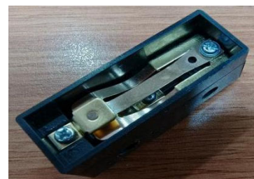
Figure 2. Internal Physical Diagram of YBLXW-5 Series Micro Switch
