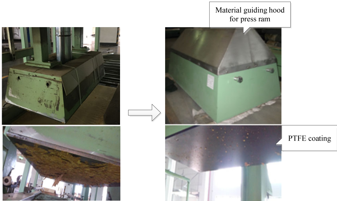
Figure 8. Optimized Structure Diagram of Press Ram
