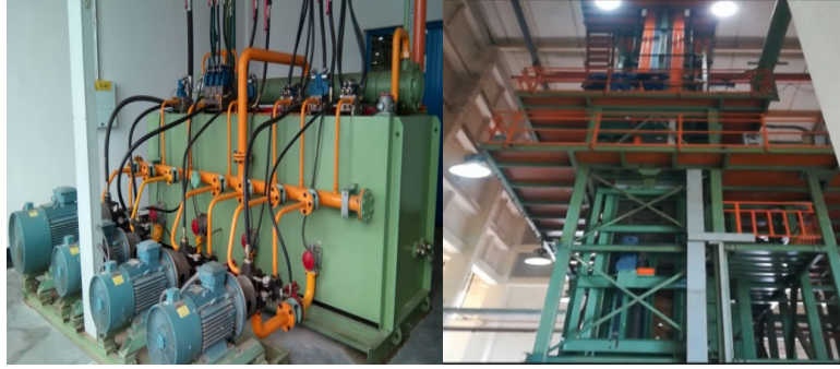
Figure 1. Double-Hydraulic Pre-Pressing and Packaging Machine of Hubei Xinye Tobacco Sheet Development Co., Ltd.
