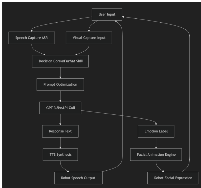
Figure 1: Outline of the model used in this study to generate emotions using GPT-3.5.
