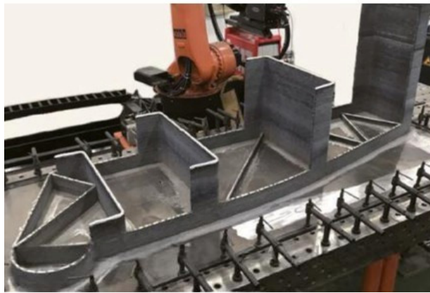
Figure 10. Thin-walled aluminum alloy parts manufactured by arc additive manufacturing [67]
