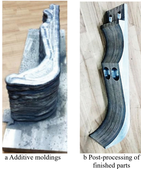
Figure 9. Pulsed GTAW Aluminum Alloy Component
