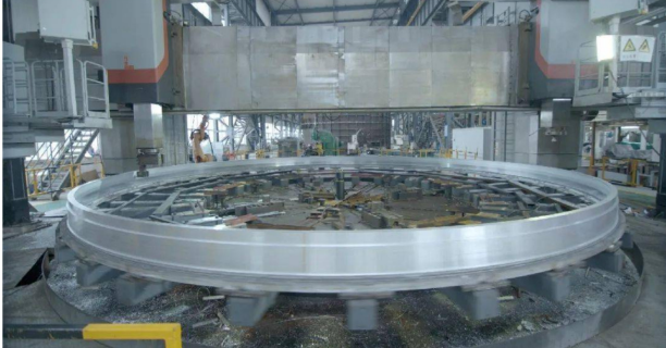
Figure 12. \varnothing 10m-class high-strength aluminum alloy heavy-lift launch vehicle connection ring prototype
