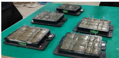
Fig 3. Physical picture of the insertion position of the steel mesh by the four-probe method.
