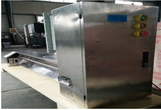
Figure 4. Physical picture of hardware system for weighing cuttings
