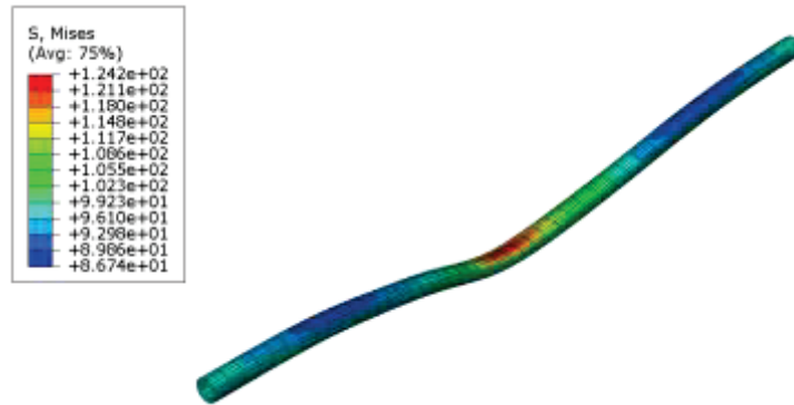
Figure 8. Maximum Mises stress cloud of pipe with 40t vehicle weight and 10km/h vehicle speed (max: 124.2MPa).
