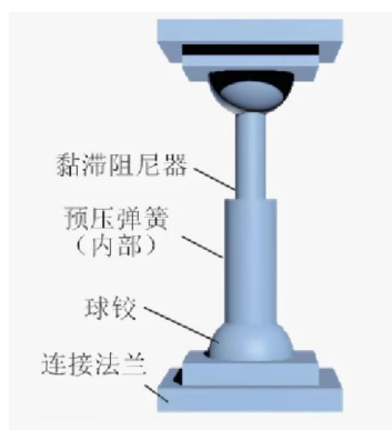
Figure 6. Negative stiffness isolation device developed by
