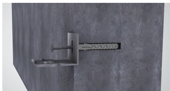
Figure 2. Installation diagram of wall fixing bracket
