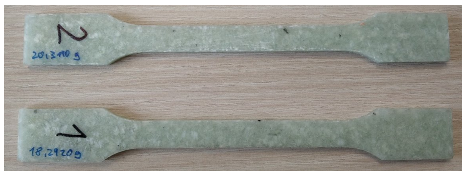
FIGURE 2. Process samples with fiberglass reinforcement, 70 % FVC (top) and 60 % FVC (bottom).
