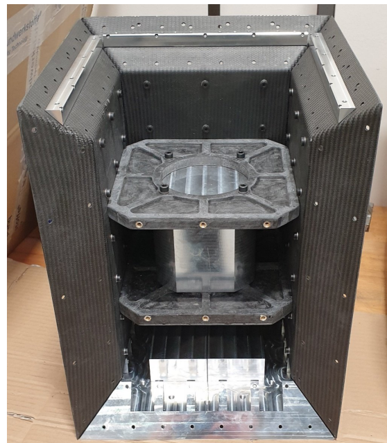
FIGURE 8. Parts in the assembly of semi-composite microsat.
