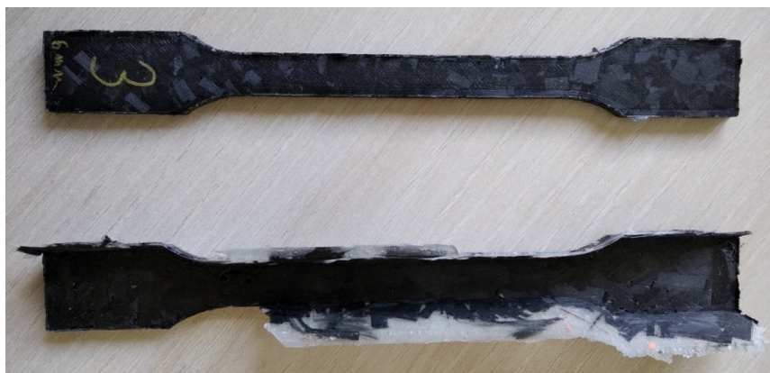
FIGURE 3. Carbon reinforced samples, 6 mm long fibres (top), 12 mm long fibres (bottom), not yet cleaned after removal from the mould.
